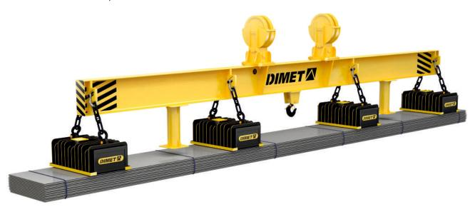
Electromagnetic spreader beam used for mild slab turning. It consists of the traverse, two special electromagnets and uninterrupted power supply system. The spreader beam significantly speeds up the slab turning process compared to stationary hydraulic devices for slab turning
