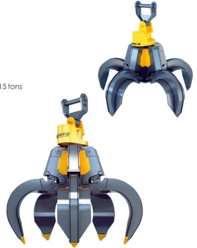
Grapple is a gripping device with 4-5 tines. Each tine is driven by a double-acting hydraulic cylinder. All the cylinders are connected to a single hydraulic circuit that coordinates the opening and closing of the tines. Due to this structure, during closing, all the tines operate with the same clamping force,
